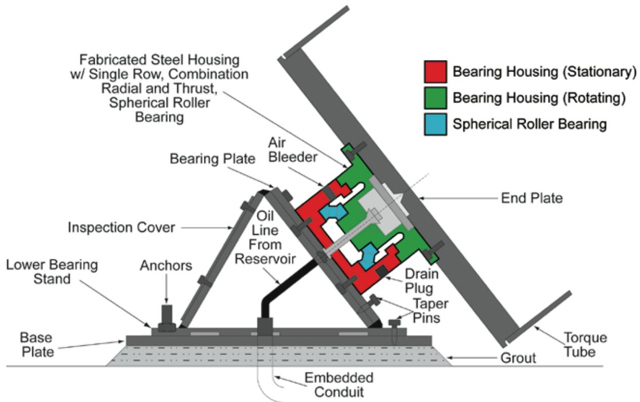
1. Combination radial and thrust spherical roller bearing
